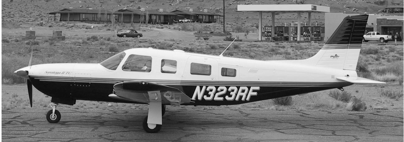
Figure 1: A Piper Saratoga II TC low-wing airplane
