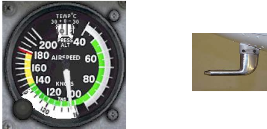
Figure 7: Airspeed indicator and pitot tube
